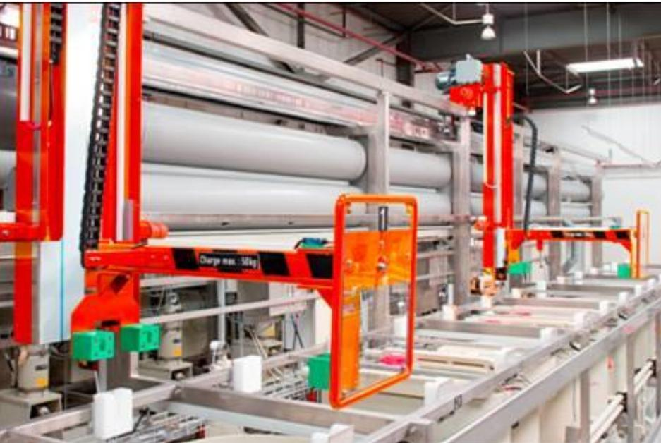
Electroplating plant for surface treatment
