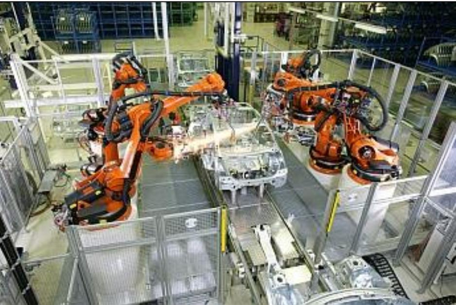
Flexible manufacturing system (Kuka)
